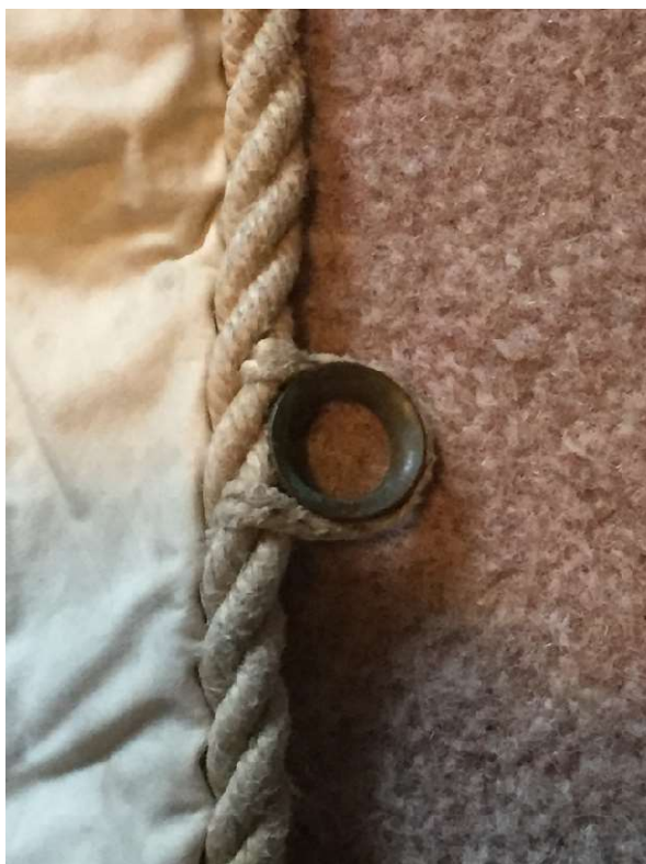
The cotton sail fabric was stitched to the luff rope, and cringles were stitched into the luff rope for attachment to the bottom of the yard..
