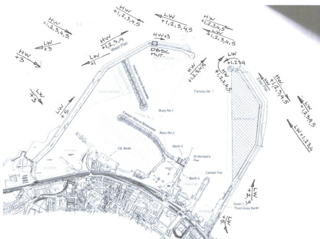
DIAGRAM OF TIDAL FLOWS AROUND DUN LAOGHAIRE HARBOUR
