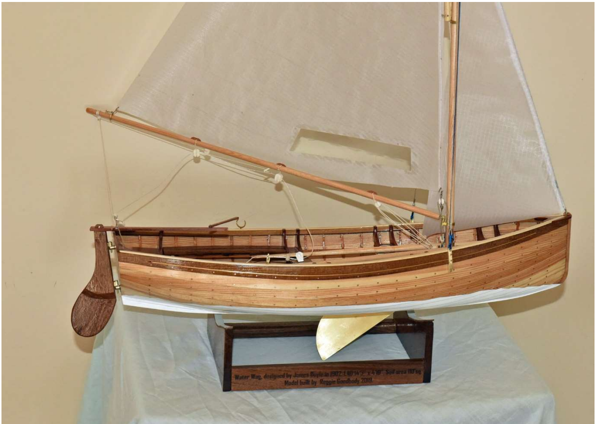
Water Wag designed by James Doyle in 1902. L&B 14'-3" x 4'-10" sail area 110'sq.
